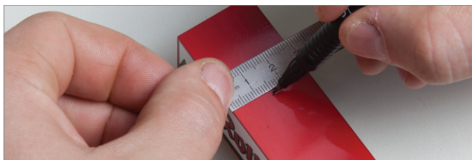
Fig. 36: Marking the position of the ultrasonic capsule
