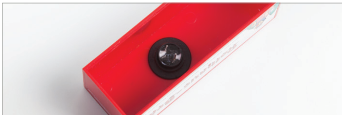
Fig. 39: Securing the ultrasonic capsule
