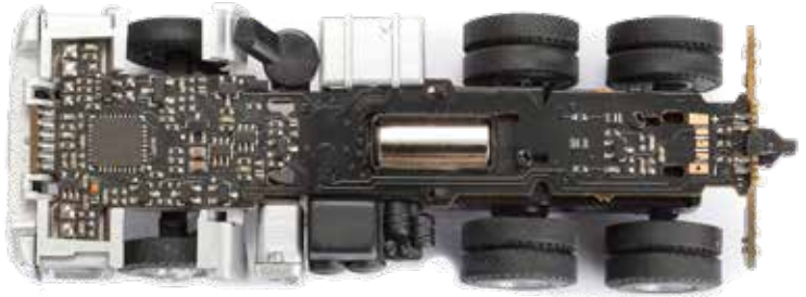
The circuit board serves as chassis.
