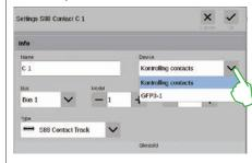
You set the device to which the feedback contact is connected in the drop-down menu "Device".
