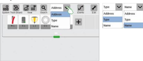
You sort solenoid items by different criteria by means of the drop-down menu on the upper edge of the item list: by the assigned address, the item designation in question ("Name") and the type of item.
