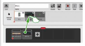
A desired locomotive or powered unit can be drawn from the locomotive list similar to solenoid items and it can be placed in the timeline.
