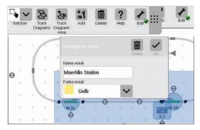
You must have selected an area in order to create an area. In this example, we are creating an area from the two-dimensional station that has been selected (see left image). To do this, open the corresponding drop-down menu with a tap of your finger on the button "Track Diagram/ Area" and select "Create area from selection" there. Give the area a name in the entry template that is turned on, select its color, and confirm with "Ok".
