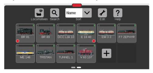
In the beginning, we recommend that you first register all locomotives with mfx decoders (see Getting Started Quickly on Page 5). This is the easiest way to fill the locomotive list (upper image) and to get started quickly.
