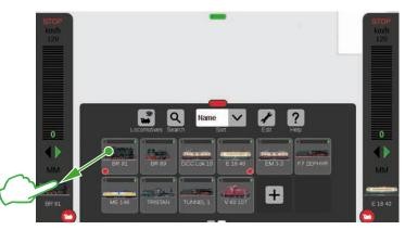
A small red dot in the locomotive list highlights the two locomotives active in the locomotive controllers.
