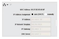
This option is available when you connect your Central Station 3 to your router with an LAN cable. Here you have the choice whether the CS3 is to obtain the necessary network addresses from the router or whether you are to enter the data manually.
