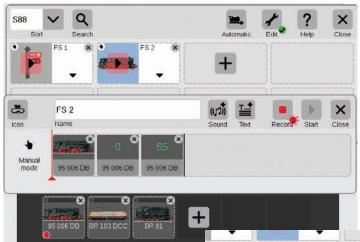
Along with the manual entry of routes and procedures, with the CS3 you can also gather these items by means of a recording function. Similar to a video camera, the CS3 records a procedure here and plays it back later.
