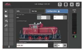
You are now in the opened tab "Info" for the locomotive settings. Even with mfx locomotives, you can change the name and the maximum speed shown on the locomotive controller – if desired.
