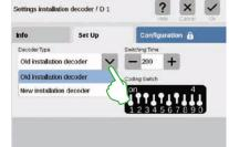
Now you have access to all of the settings in the tabs "Info" (name, address, type, protocol, and decoder) (left image) and "Set Up" (type of decoder and switching duration) (right image).
