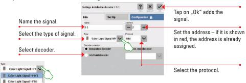
You determine the type of signal by means of a drop-down menu that you open up with a tap of your finger. Different signal variations are there ready to be selected.
