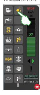
The functions are switched by tapping on the function symbols. For example, in the image to the left the light, coupling/ uncoupling, the whistle, and the blowers are being activated.
