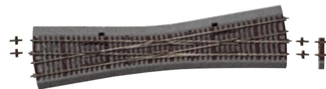
Simple diamond crossing with slips 10 deg., „English“ design with inside tongues, for manual operation, length 345mm, turnout radius 959mm, crossing angle 10 deg. With bedding. Two distancers D2 and D8 are enclosed for length compensation. Matching electric drive 42620 (2x) or 42624 (2x).
