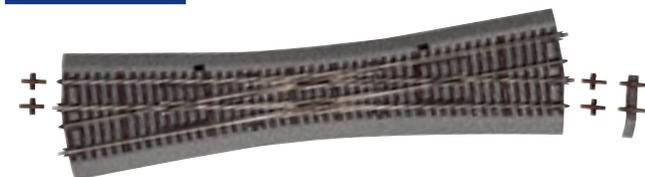
Double-slip switch DKW 10, „English“ design with inside tongues and manual operation, length 345mm. Frog angle 10 deg., turnout radius 959mm. With bedding. Two distancers D2 and D8 are enclosed for length compensation. Matching electric drive: 42620 (2x) or 42624 (2x).
