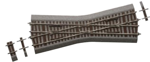
Crossing K15, length 230mm, crossing angle 15 deg.; the frogs can be polarized with a 10019 relay, crossing can be integrated in a track protection arrangement like a normal magnetic item. The crossing railway tracks are not electrically separated. For the installation of diagonals, two off D4 and one off D12 are enclosed. With bedding.
