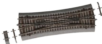
Double-slip switch DKW 15 version „Baeseler“, with outside tongues. Length 230mm, crossing angle 15 deg., effective turnout radius 1050mm. Polarized ex works due to the electrical requirement of this diamond crossing with slips. For installation of diagonals, two off D4 and one off D12 are enclosed. With bedding. For Art. No. 42546: Matching electric drive 42620 (2x) or 42624 (2x).
