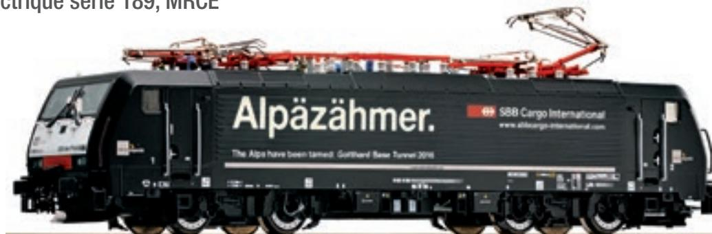
Motor with flywheel. Drive on four axles. Triple headlights that change over with the direction of travel.
