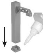
*Now glue the pre-assembled mast to the ground plate.*
