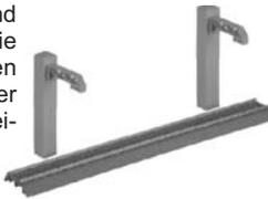
*Then install the other masts in the same way. The distances between the individual poles should not exceed 25 cm in straight lines and 20 cm in curves.*
