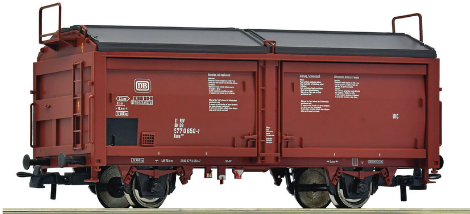
Sliding roof/sliding wall wagon, type Tims, of the Deutsche Bundesbahn.
