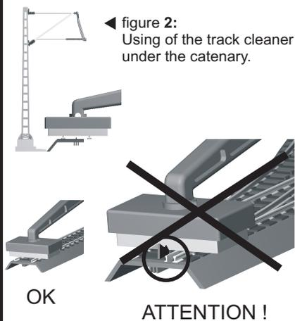
**figure 3:** Attention at three rail turnouts
